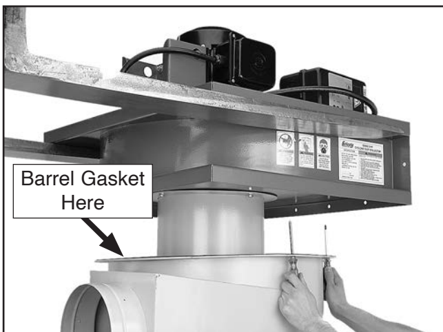
Figure 18. Aligning mounting holes.
