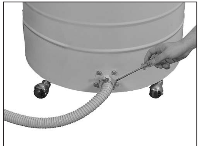
Figure 39. Connecting vacuum hose.
