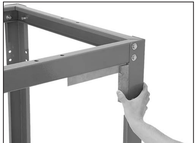
Figure 12. Example of squaring stand assembly before tightening stand hardware.
