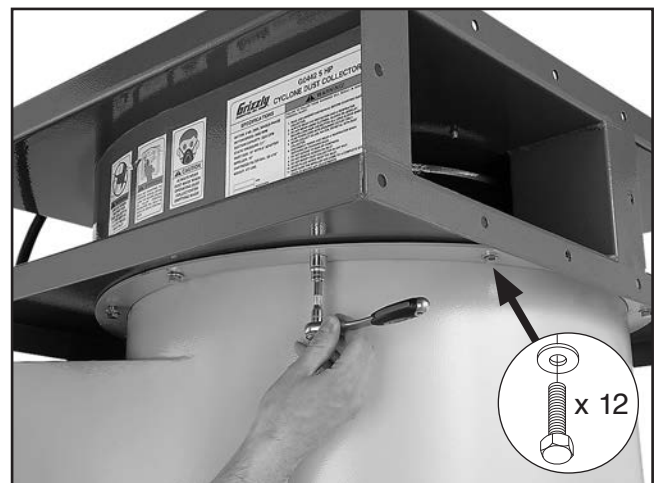
Figure 20. Securing blower on intake barrel.
