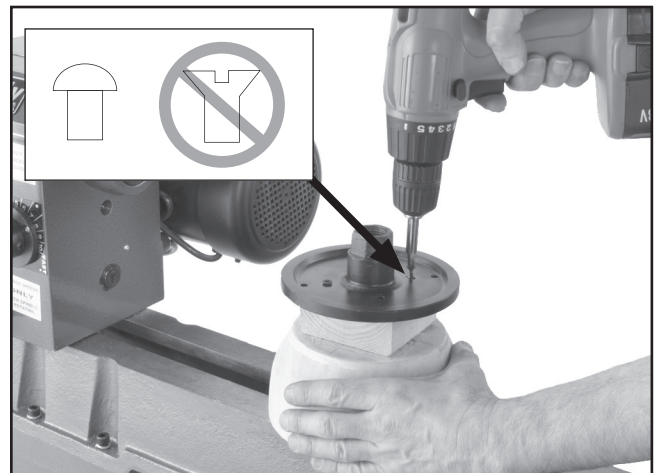
Figure 28. Mounting a typical faceplate to a backing block, which is glued to the workpiece.
