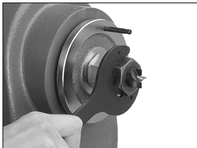
Figure 16. Removing spur center.
