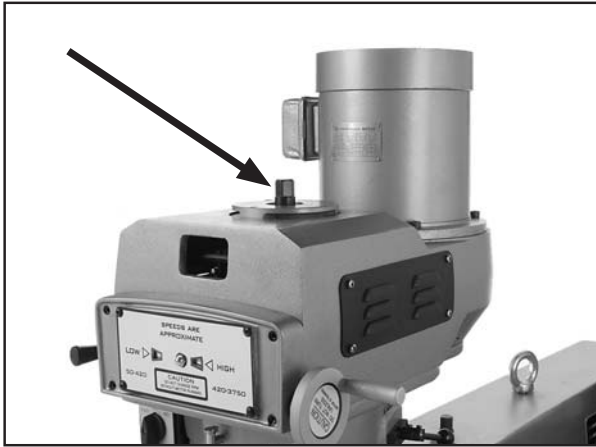
Figure 46. Drawbar inserted through the top of the spindle.
