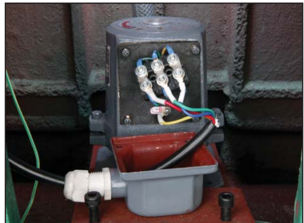
Figure 76. Coolant pump wiring.
