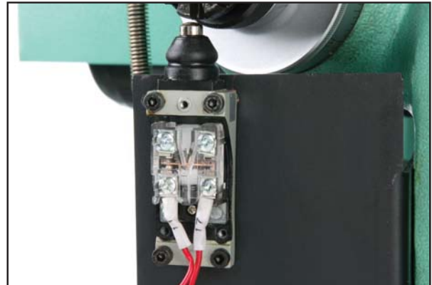
Figure 80. Vertical crank safety switch wiring.
