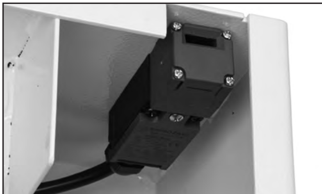
Figure 34. Upper door limit switch.
