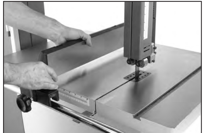
Figure 25. Example of installing fence onto rail.
