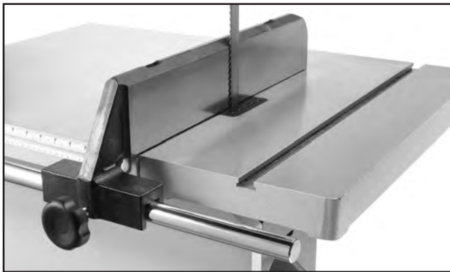
Figure 41. Example of fence flush with blade.
