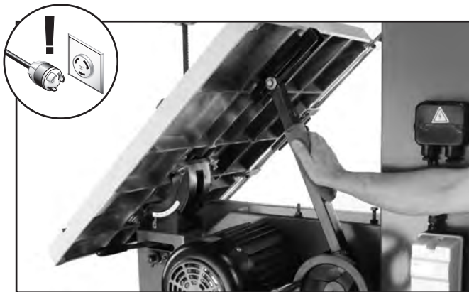
Figure 72. Example of lubricating table tilt rack and pinion assembly.
