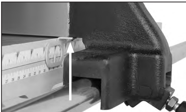
Figure 42. Fence pointer adjustment screw.
