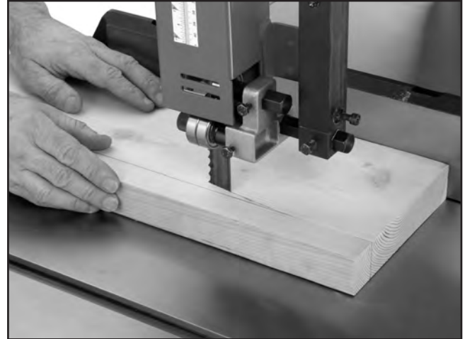
Figure 59. Blade leading away from line of cut.
