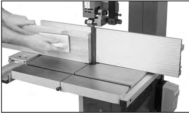
Figure 58. Example of resawing lumber.
