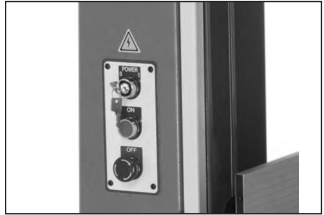
Figure 32. G0568 switch disabling key and ON/OFF switch.
