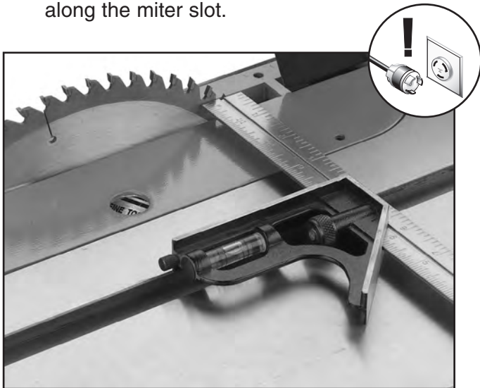
Figure 76. Example of adjusting blade to miter slot.
