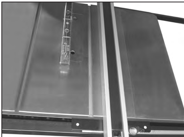
Figure 82. Example of fence aligned parallel to miter slot.
