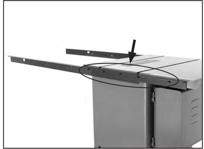
Figure 11. Rear rail installed.
