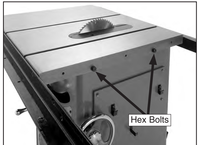
Figure 12. Hex bolts installed.
