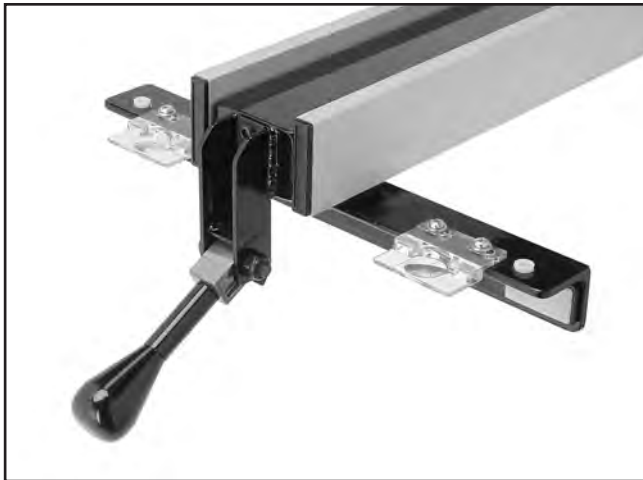
Figure 32. Fence knob installed.
