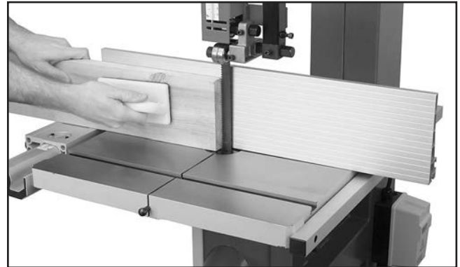
Figure 53. Example of resawing lumber.
