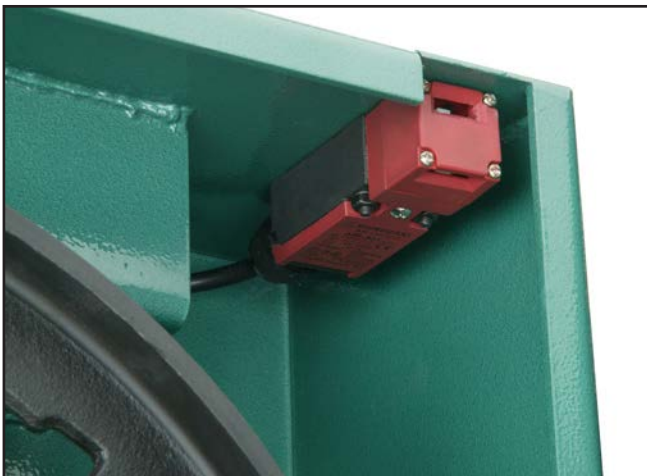
Figure 89. Wheel cover limit switch.
