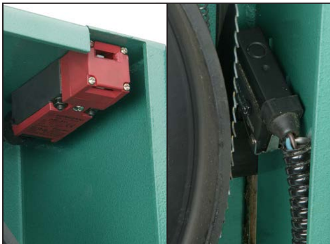
Figure 84. Wheel cover limit switch (left) and foot brake switch (right).
