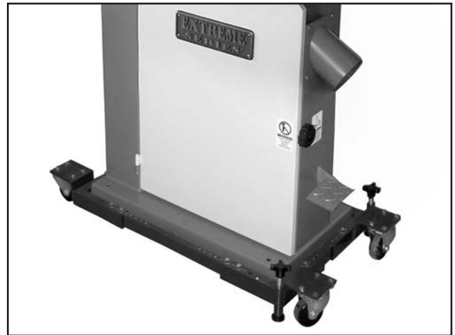
Figure 12. Bandsaw mounted on D2058A mobile base.
