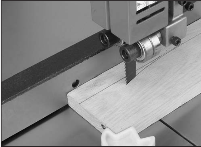
Figure 50. Example of blade leading away from line of cut.
