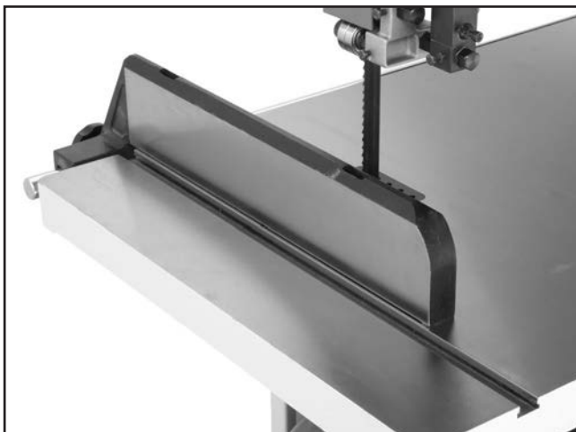
Figure 39. Example of fence square with miter slot.
