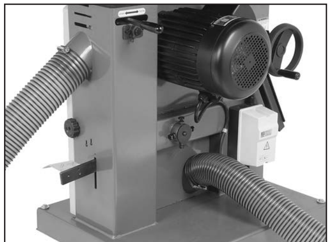
Figure 19. Dust hoses attached to dust port.
