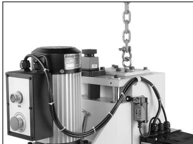
Figure 8. Boring machine attached to lifting equipment.
