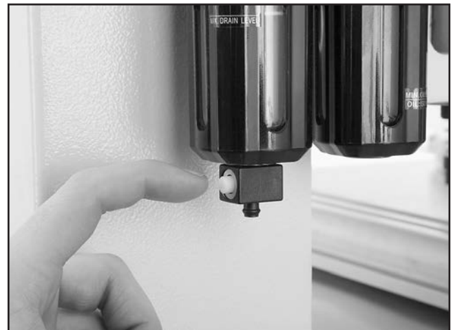
Figure 34. Release water from the air filter reservoir.
