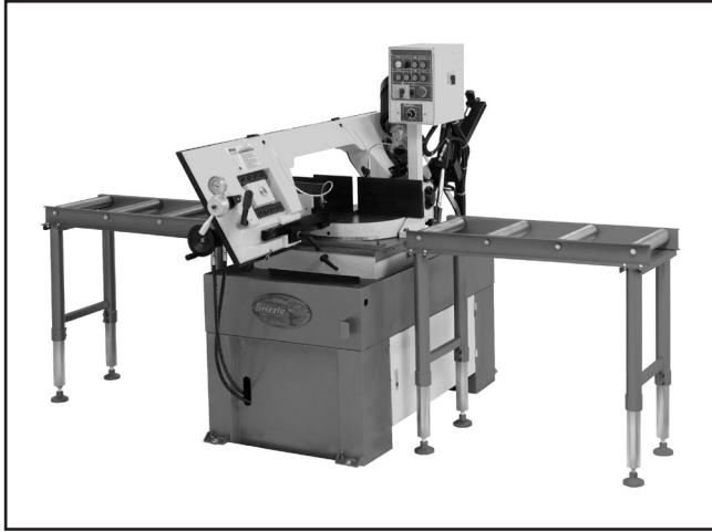
Figure 15. Positioning roller tables.
