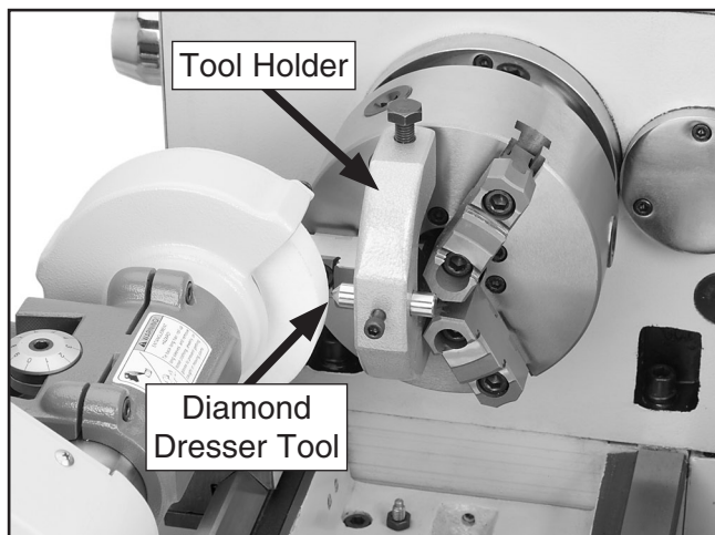
Figure 25. An example of the diamond dresser tool and holder mounted on a chuck jaw
