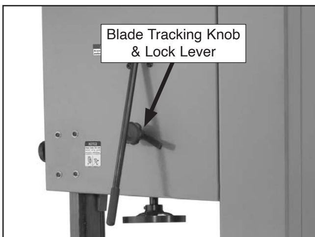
Figure 16. Blade tracking knob and lock lever.
