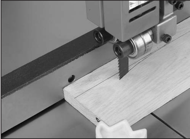
Figure 69. Example of blade leading away from line of cut.
