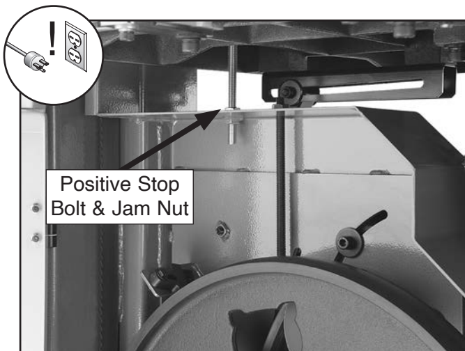
Figure 18. Positive stop bolt and jam nut.
