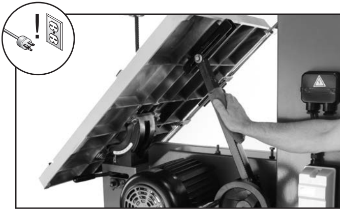
Figure 64. Lubricating table tilt rack and pinion assembly.
