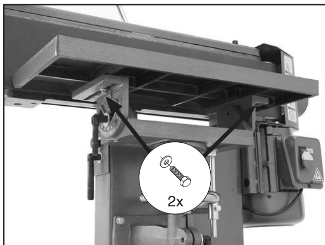
Figure 23. Work table installed.
