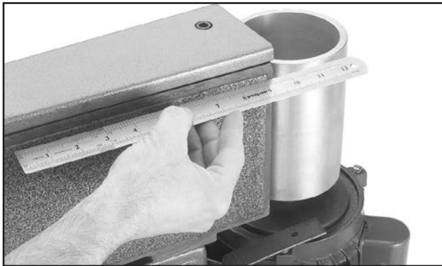
Figure 54. Example of checking top of platen-to-roller.
