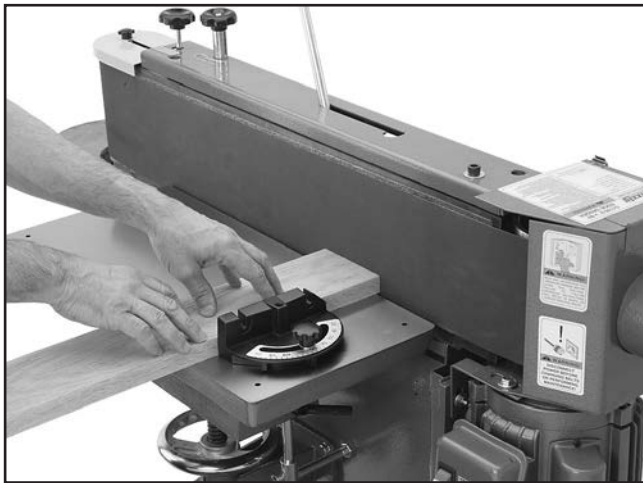
Figure 38. Typical end grain sanding method using miter gauge.
