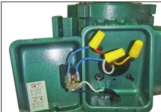
Figure 59. G1140 motor wiring (prewired 220V).
