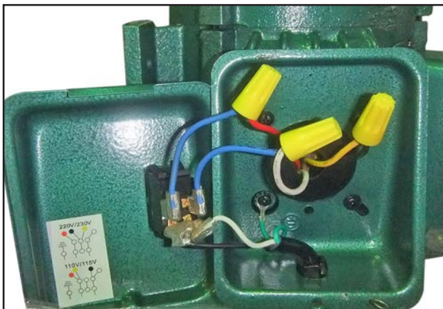
Figure 61. G1531 motor wiring (prewired 220V).
