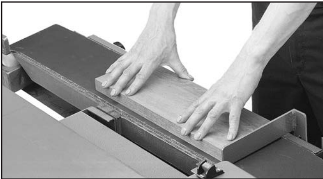
Figure 40. Example of face sanding method.
