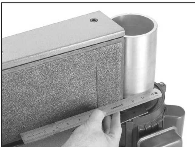
Figure 55. Example of checking bottom of platen-to-roller.
