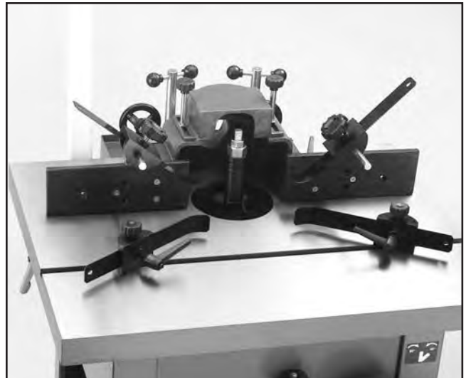
Figure 21. Overview of hold-downs in place.
