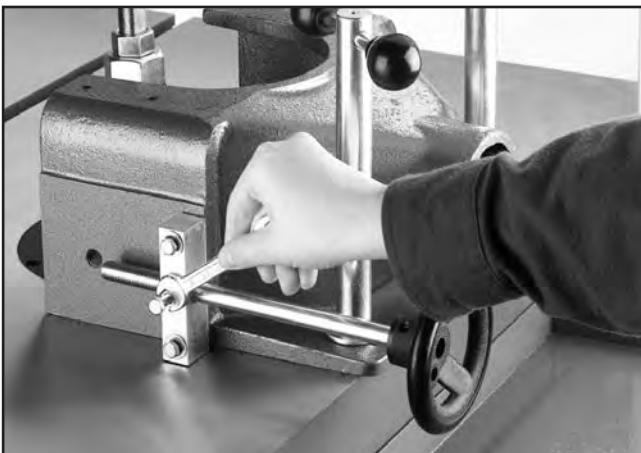
Figure 14. Tightening bolt into shaft groove.
