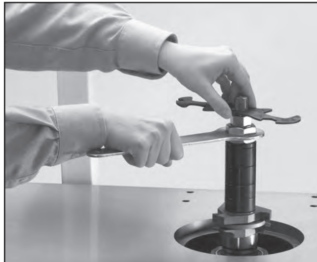
Figure 29. Tightening spindle nuts.
