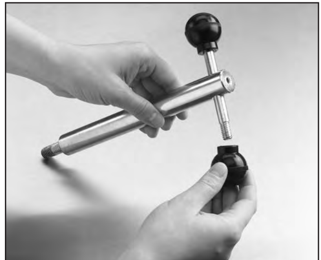
Figure 11. Round knobs onto bar.
