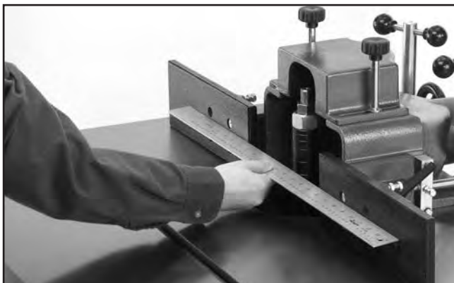
Figure 25. Aligning fences with straightedge.
