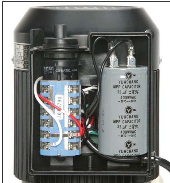
Figure 23. Motor switch and capacitor.
