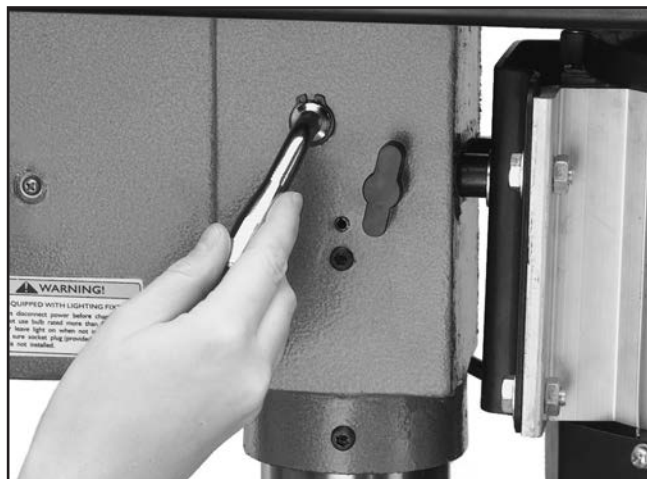
Figure 29. Using the belt tension lever.
