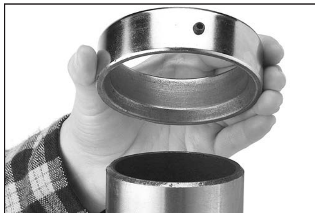
Figure 16. Correct column ring orientation.
