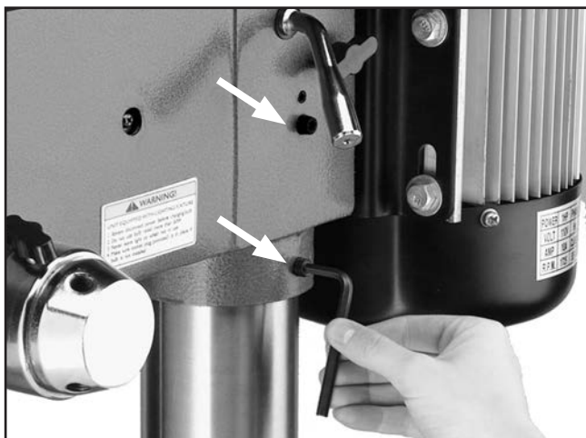
Figure 20. Securing headstock to column.
