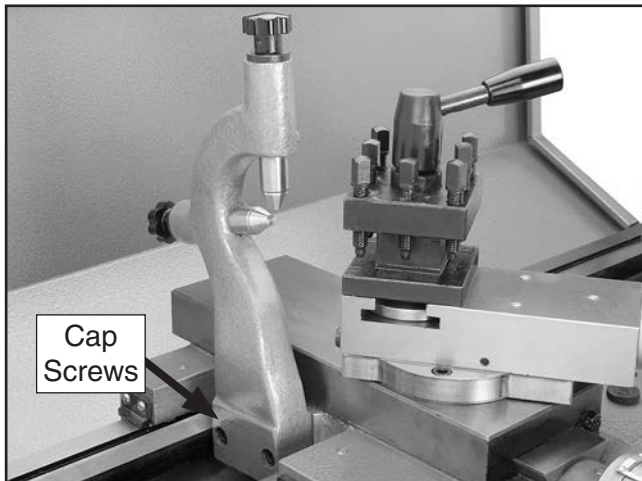
Figure 44. Follow rest mounted on the saddle.
