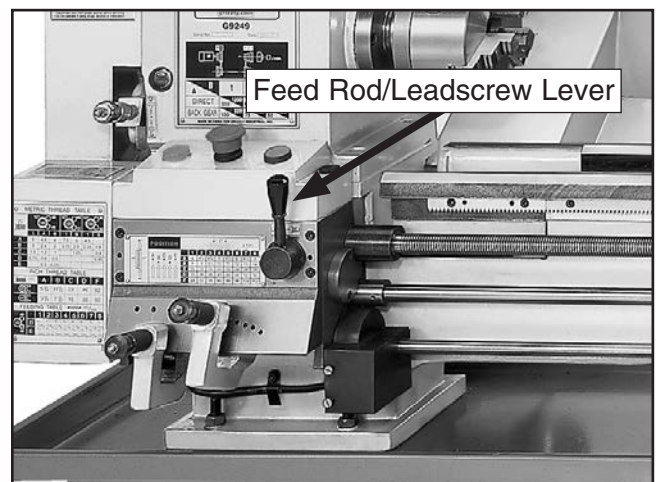
Figure 16. Feed rod/leadscrew lever in center (neutral) position.
