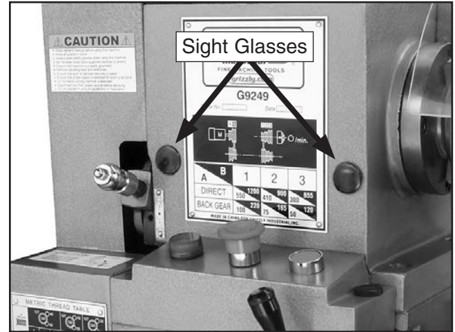
Figure 79. Spindle bearing reservoir oil sight glasses.
