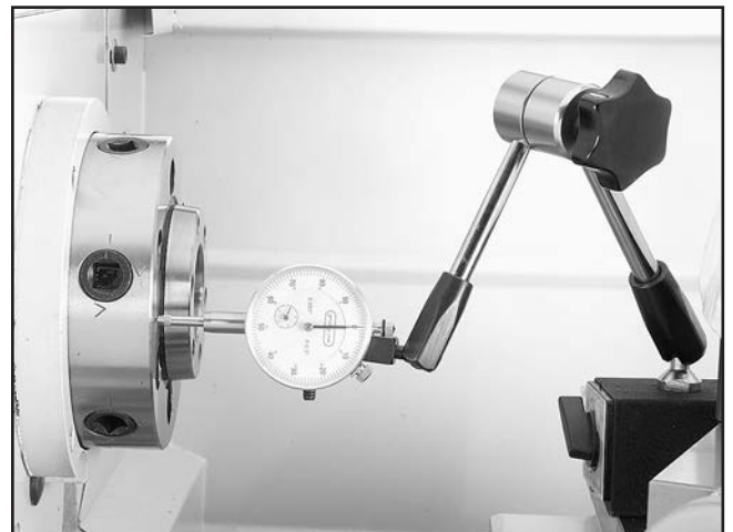
Figure 104. Example of test indicator setup.
