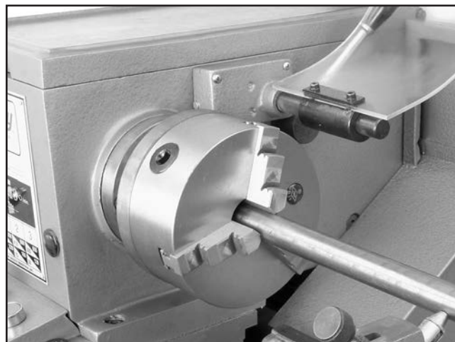
Figure 26. Example of workpiece firmly held in the center of the 3-jaw chuck.
