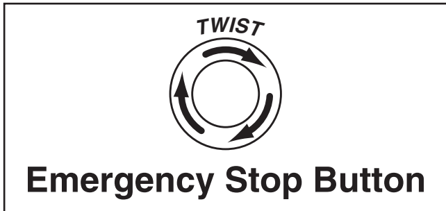
Figure 17. Resetting the emergency stop button.
