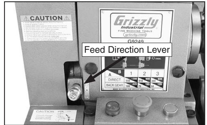
Figure 23. Feed direction lever.
