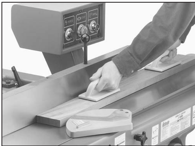
Figure 40. Example of surface planing with the jointer.
