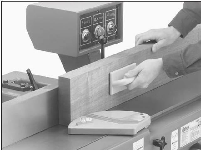
Figure 42. Example of edge jointing operation.
