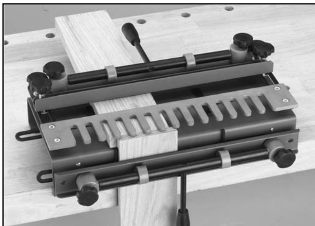
Figure 18 shows the dovetail jig set up for use. The inside faces of the boards are showing.
