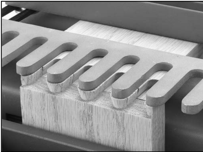
Figure 8 shows correct alignment when clamping pressure is properly adjusted.
