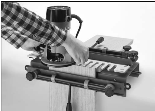
Figure 19 shows the dovetail jig in use.
