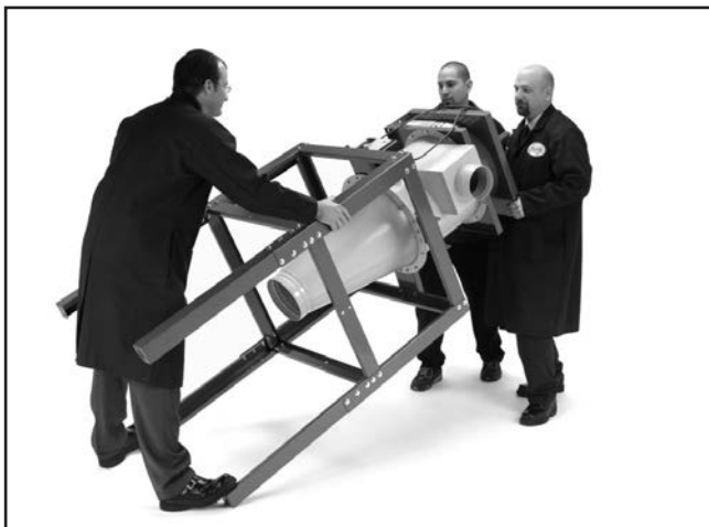
Figure 14. Lifting the assembly upright.
