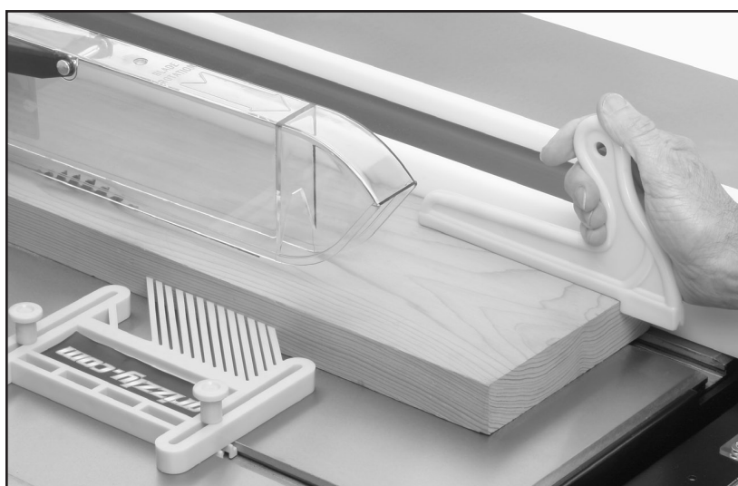
Figure 2. Using the push block.
