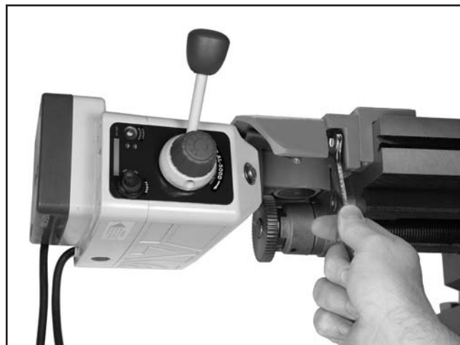
Figure 8. Installing the power feed and mounting bracket assembly onto the table bracket.
